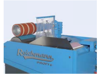
Comfortable change from stone to belt due to pneumatic lifting device
